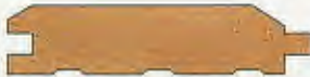
MVG-20 3/4 x 2-3/4 FACE MVG-30 3/4 x 3-1/4 FACE MVG-40 3/4 x 4-1/4 FACE MVG-50 3/4 x 5-1/4 FACE
